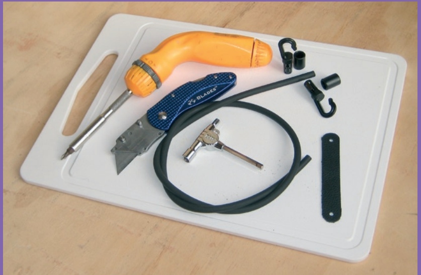
▲ If mounting internally, you'll need some simple tools to fit the Shu: a knife to cut the rubber, a screwdriver to unscrew the lug screws and a drum key to remove the batter head.
